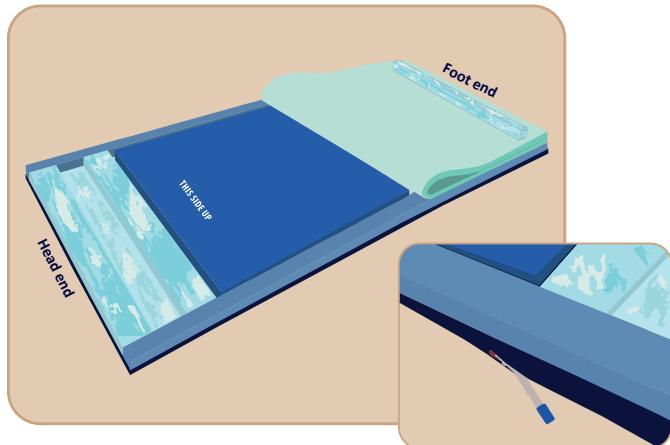
2. The top plate can be opened at the head end. Underneath is the air-cell circuit in a cover.
